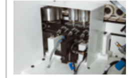
Otomatik Ayarlı Baskı Merdanesi Automatically Adjusted Pressure Rollers
