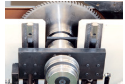
Linear Yataklı Ana Testere Ünite Hareketi Main Saw Blade Unit Movement via Linear Guide
