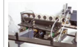
Otomatik Ayarlı Ön Siper Automatically Adjusted Fence
