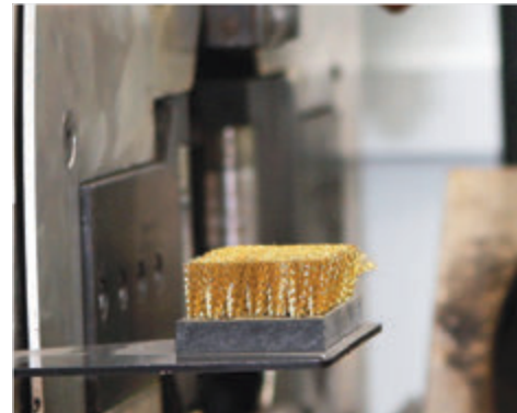
■ This is used for automatic cleaning of the nozzle that was contaminated during the cutting processes of materials. (S)
