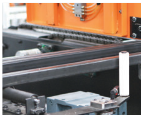
■ Thanks to the profile separation system, profiles on the loading chain are referenced and it is ensured that a single profile is loaded at a time.
