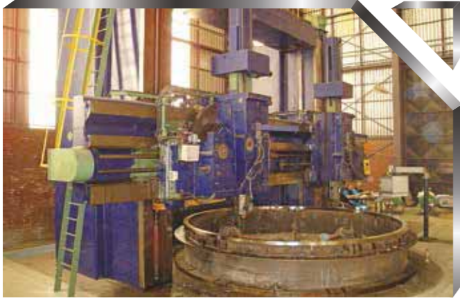
CNC Dik Torna Ø: 5.850 mm, h : 3.400 mm CNC Vertical Lathe
