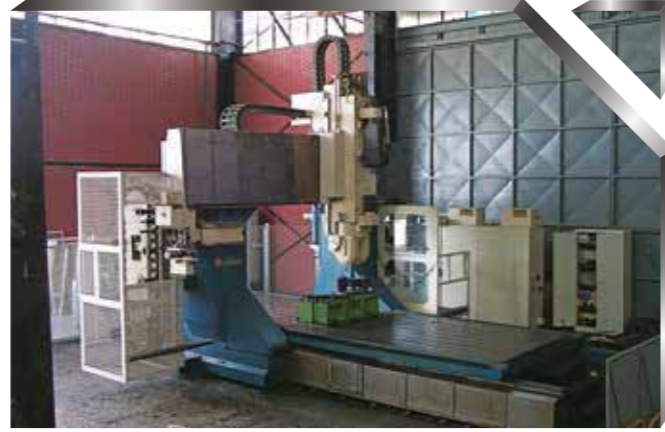
5 eksenli / 5 axis TOS Kurim FRFQ 2000 x:4.000mm, y:2.800mm, z:1.100mm
