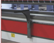
● Lineer kızaklı kayan ön kollar Support arm for sliding
