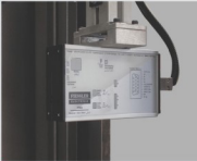
● Ön Laser parmak koruma Front laser finger protection
