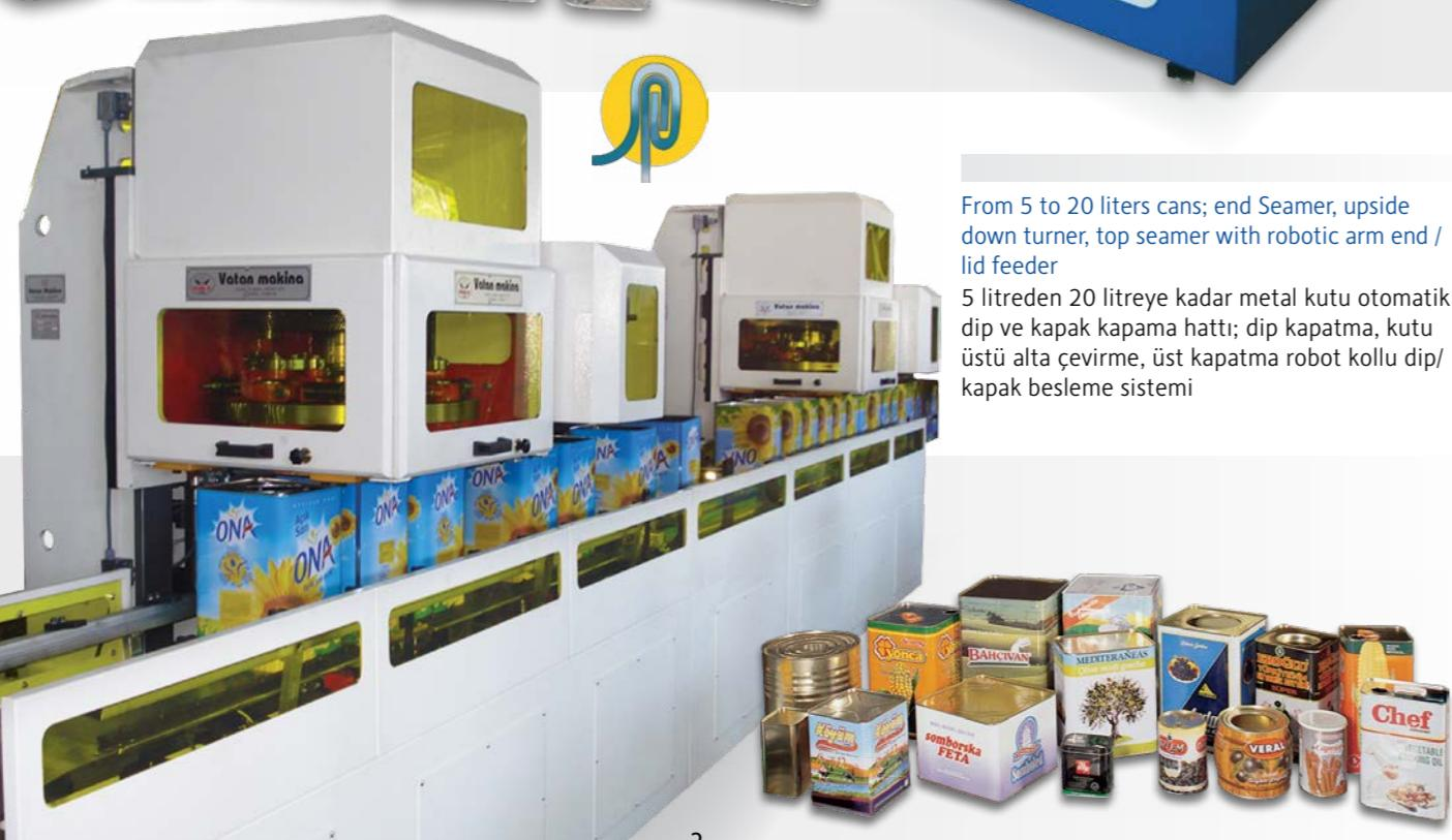
From 5 to 20 liters cans; end Seamer, upside down turner, top seamer with robotic arm end / lid feeder
