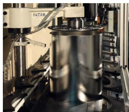
Indexing; detecting & positioning of welding
