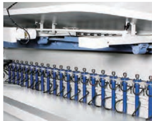
■ Anti twist system prevents twisting of sheet metals by holding the sheet metal being cut against top blade moves during cutting period (O)
