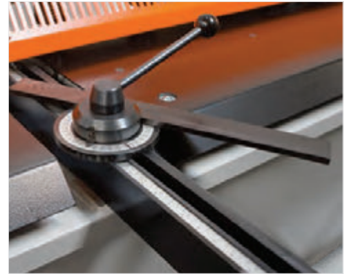
■ High precision, easy cutting at angled cutting thanks to angle adjusted T-square (O)
