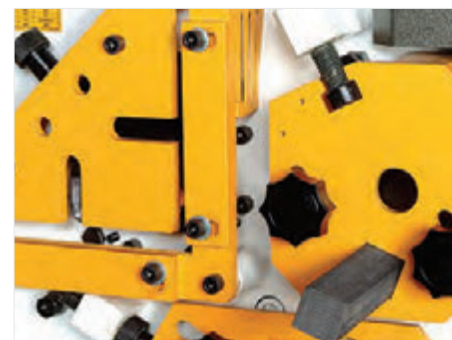
■ Bar cutting station
