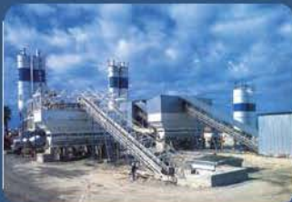
Ağrega Yer Besleme Sistemleri Aggregate bunker belt conveyor feeding systems
