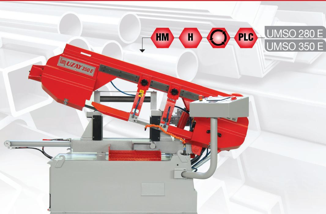
Scissor type, full automatic bandsaw machine. The machine has PLC programming, the materials feeding is done with motorised rollers of the vice system. Length measurement is done via encoder. Good for high production shops with straight cutting requirements especially for automotive and spare parts manufacturers.
