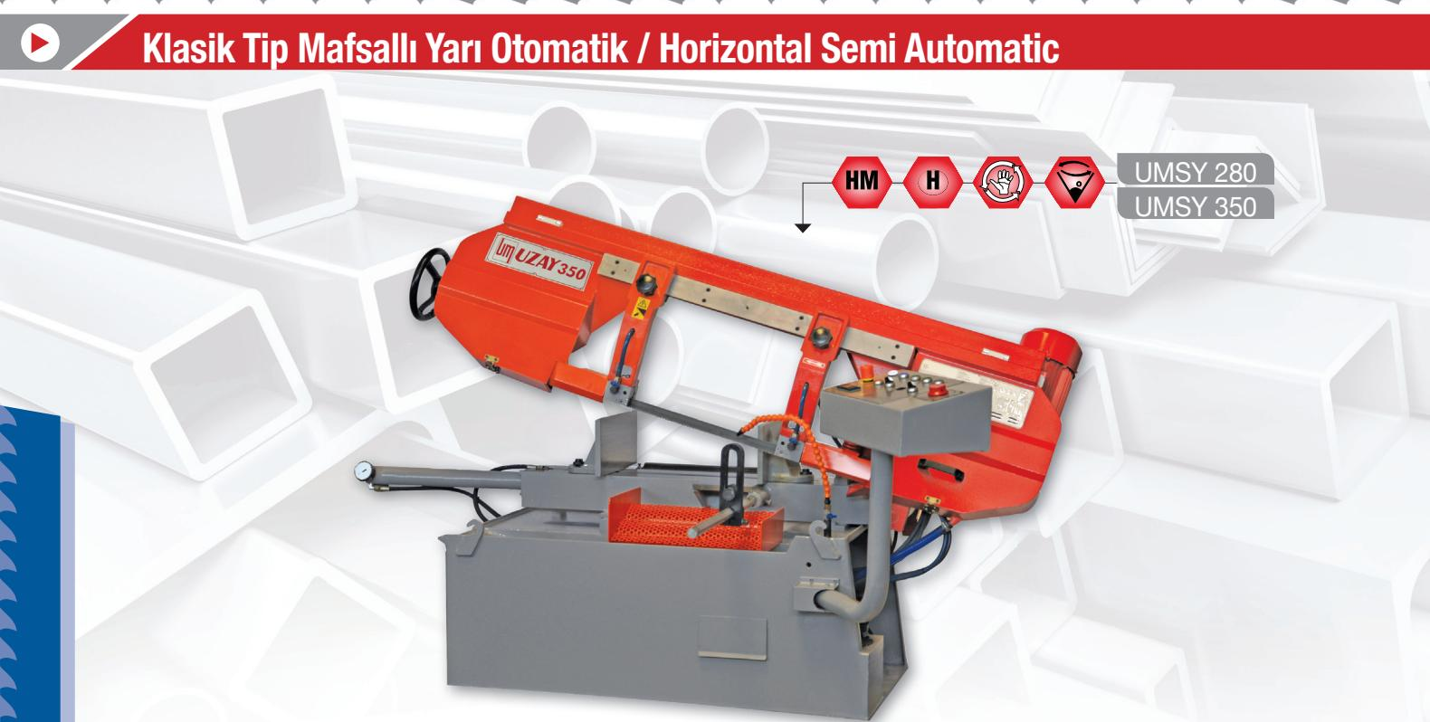
Scissor, semi automatic bandsaw machine. The material positioning is done manually. Good for workshops having single cuts. Also angular sawing is available by swivel vice jaw.
