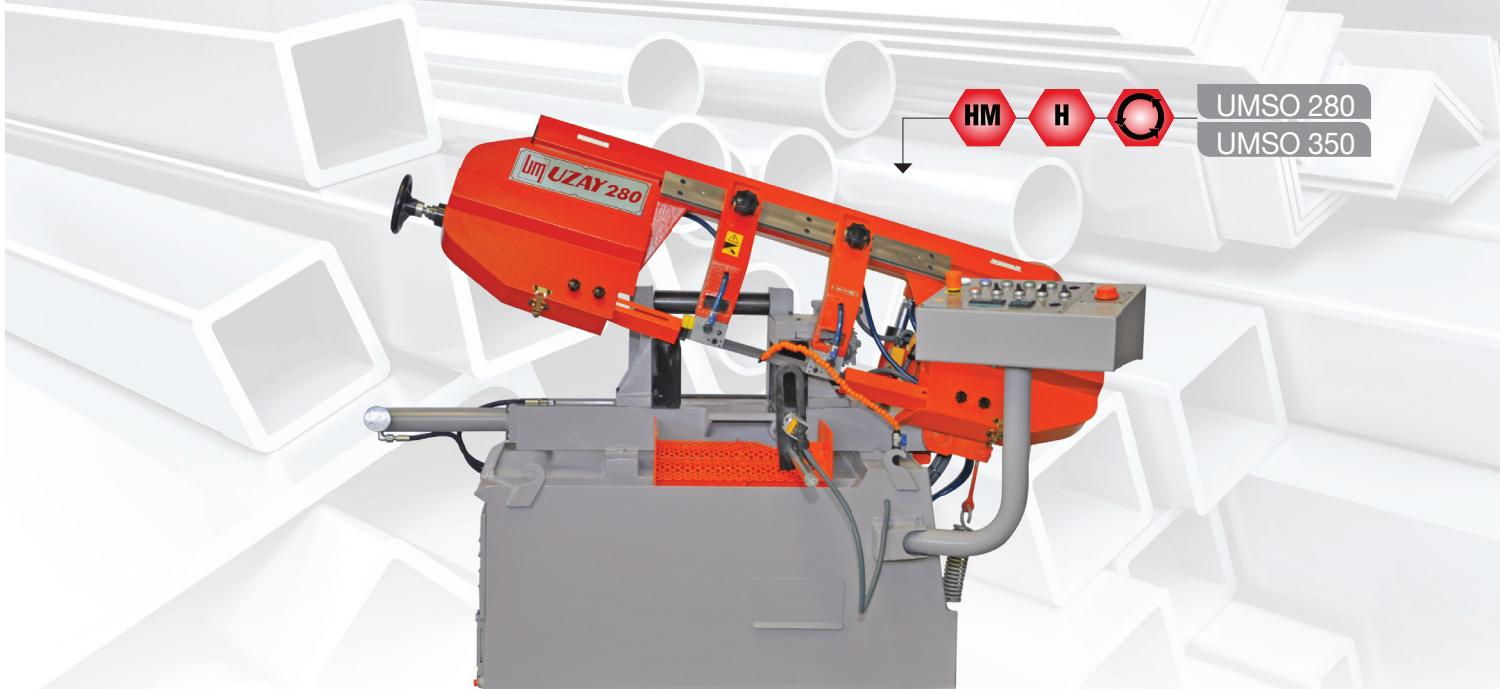
Scissor type, full automatic bandsaw machine. The length is preset via switch lengthstops. The materials feeding is done with motorised rollers of the vice system. Good for high production shops with straight cutting requirements.
