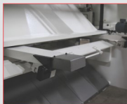
● Ball screw arka dayama 750 mm Ball screw back gauge 750mm
