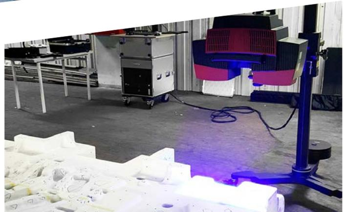
ATOS 3D Scanning and Measuring System for dimensional control of patterns and castings
