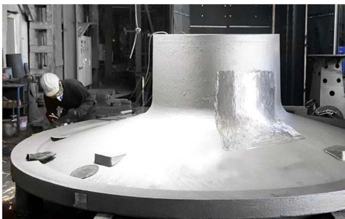
Magnetic & Dye penetrant testing for castings
